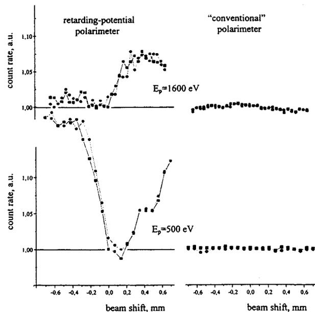
FIG. 4. Normalized count rate vs beam shift from the axis of the Mott polarimeter (axis Z; see Fig. 3) for two primary electron energies, 500 and 1600 eV.
