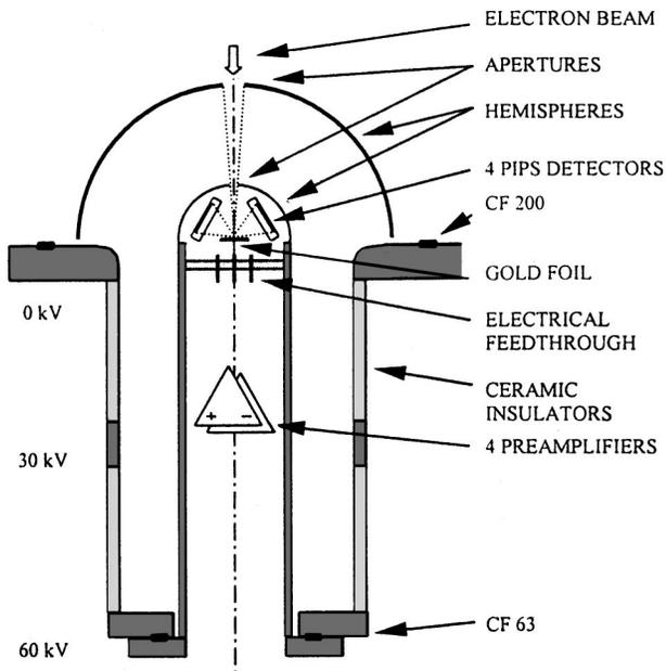
FIG. 1. Schematic of the spherical field-free polarimeter.
