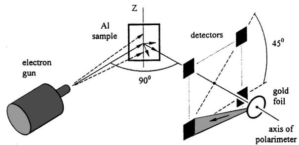
FIG. 3. Scheme of the experiment.
