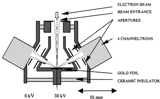
FIG. 2. Schematic of the conical retarding-potential polarimeter.
